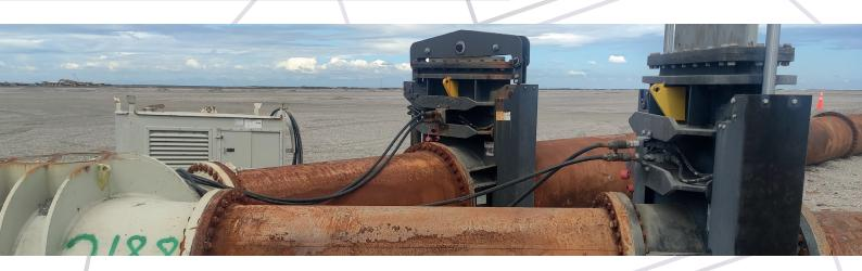
These valves are used on shore. They are robust enough for rough handling and they are easy to transport. The shore valves enable the closing of the discharge pipes while maintaining pre-designed pressure.
