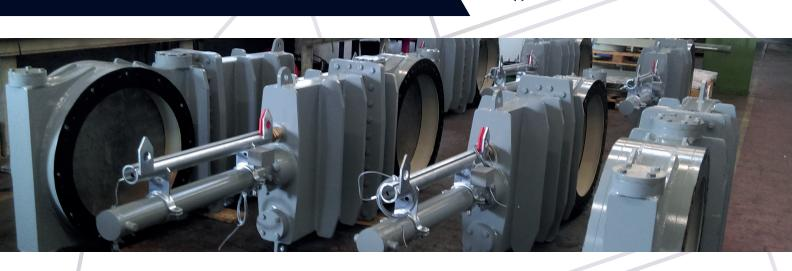
Our regulating valves are used on dredgers. The gate can be controlled in such a way that the flow can be regulated. By controlling the flow the dredging process is optimized.
